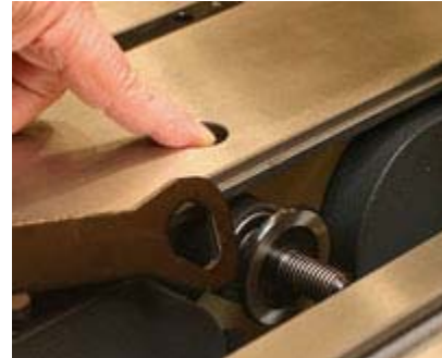
Blade changing on the ProShop saw requires the included blade wrench and a single finger to depress the arbor lock.
